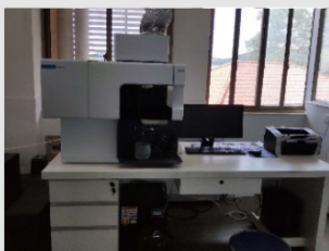
电感耦合等离子体发射光谱仪 ICP-OES-Inductively Coupled Plasma Optical Emission Spectrometer , Thermo Fisher
