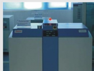
荧光光谱仪 X-Ray Fluorescence Analyzer
